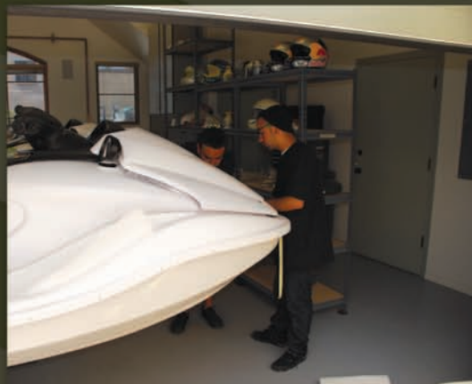
(Right) After all OEM stickers, paint, trim and traction mats were stripped away, the entire upper deck was sanded, sanded, and re-sanded, then painted with a white base. As C-Wood likes to put it, "Preparation is extremely time consuming – when done correctly."
