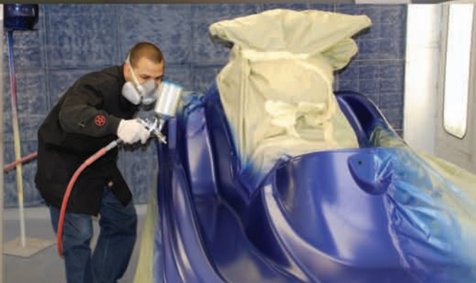
Although they can't reveal all of their top-secret painting techniques, we were able to show you this really cool shot of David, one of Airtrix's painters, laying down a coat of metallic blue paint. Every color used – silver, blue, red and yellow – is specially prepared and mixed to meet Red Bull's stringent standards.
