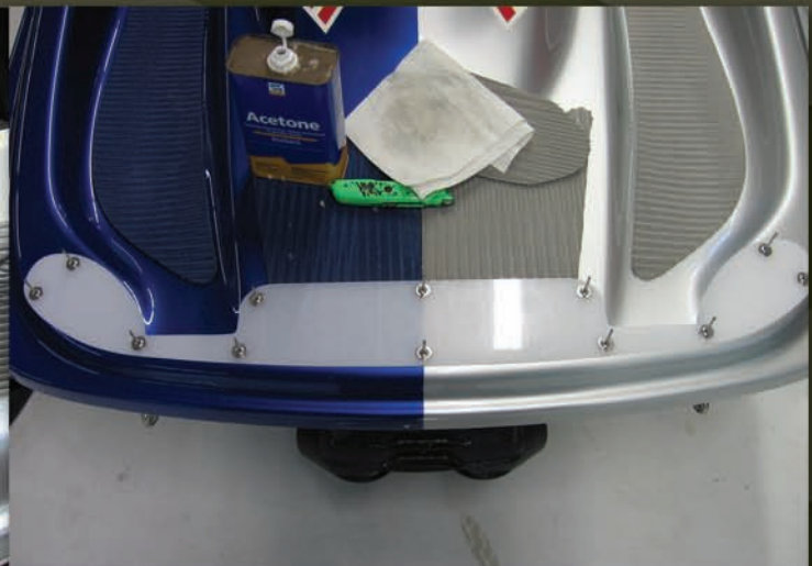
Due to the rough conditions expected in the surf, Slattery rivets a precut polypropylene sheet to the back deck, where the board will mate with the craft. The sheet is approximately the same hardness rating as the rescue board's nose cone, which will minimize wear and tear and keep the board from ruining the paint – or one component from wearing down another. Occasional replacement of a nose cone or poly sheet is easy, when compared to potentially ruining a one-of-a-kind paint job.
