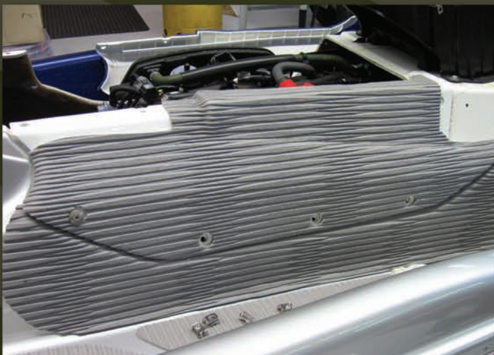
Honda's removable engine-access panels are a dream – unless you're the one tasked to cover them with EVA padding. The side panels' traction padding must be carefully cut and applied in order to match the surrounding padding's striations and to provide a watertight seal once the panel is fastened back into place. Since the EVA material doesn't absorb water, its application supercedes that of the original foam sealing trim.
