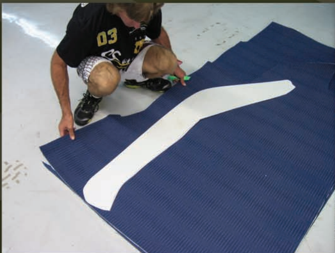
Once inside, the Hondas are stripped completely bare – again. Mike Slattery, seen here using a template to cut out some EVA traction mat, prefers to start working from the inside out, starting with the inner EVA footwell and gunwale traction pads, then progressing to the rescue board attachments and safety straps, and ultimately finishing off with the over-the-rail gunwale pads.
