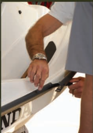
(Left) HSA's Mike Slattery helps carefully remove the remaining trim and side molding from the Aquatrax's bondline. All three craft had to be towed to Airtrix in Santa Barbara, California, and completely stripped down – naked as a newborn baby. Everything from major body parts to the tiniest nuts and bolts needed to be removed.
