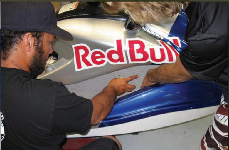
Scotty Martinson, of Channel Islands Surfboards and Al Merrick, helps Slattery mark and trim the EVA pads. In addition to fitting the contoured dimensions of the upper deck, the EVA material must be carefully chosen and the colors approved by Red Bull. After finding the perfect fit (and being careful to follow the blue and silver lines of the Airtrix paint job), a heat gun is used to aid in installation. Without it, the EVA is simply too stiff to properly contour to the curves, and the process becomes much more difficult.
